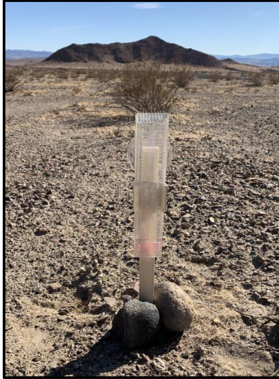
Figure 12. Rain gauges were randomly placed throughout the landscape to capture supplementary precipitation data. Gauge contains mineral oil to slow evaporation of precipitation and antifreeze to prevent freezing of precipitation. Photograph taken by S. Doyle, USGS.
